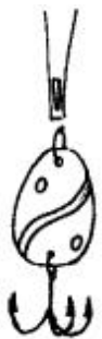
Lure made from a thrift store spoon: cut off the handle and file smooth.
