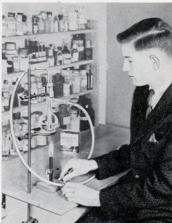
Converting a liquid oil into a solid fat, by the process used in making vegetable shortening. The apparatus is shown below
