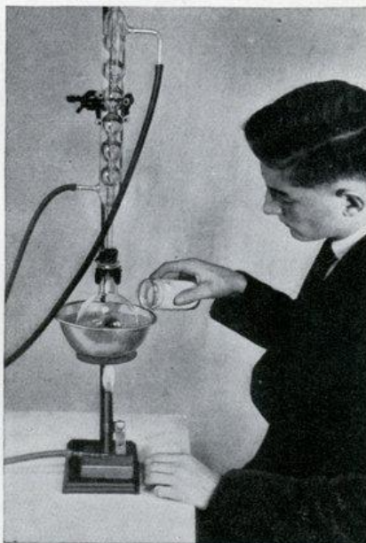
Hydroquinone, added to a vegetable oil used as a heating bath, will keep the oil from becoming rancid. Left, making a rubber substitute by heating sulphur and linseed oil
