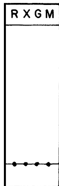
FIGURE 1-1 Plastic TLC slide with spots of the three dyes and the mixture applied. Keep the spots applied small.
