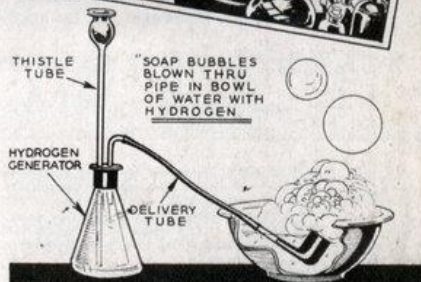
Many experiments can be performed with the Hydrogen gas generator described on opposite page. Above is shown model airship constructed of light rubber being inflated with the gas. Pipe connected to generator will blow floating soap bubbles.
