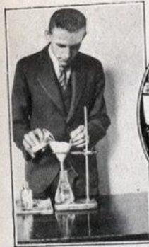
Hydrogen Peroxide, a common household antiseptic, can be prepared by mixing dilute sulphuric acid with barium dioxide. The resulting milky liquid is cleared by filtering. Before using test the solution to determine whether or not it will successfully bleach cloth.
