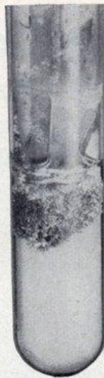
Beautiful crystals of pure silver form a treelike growth before your eyes in this striking test
