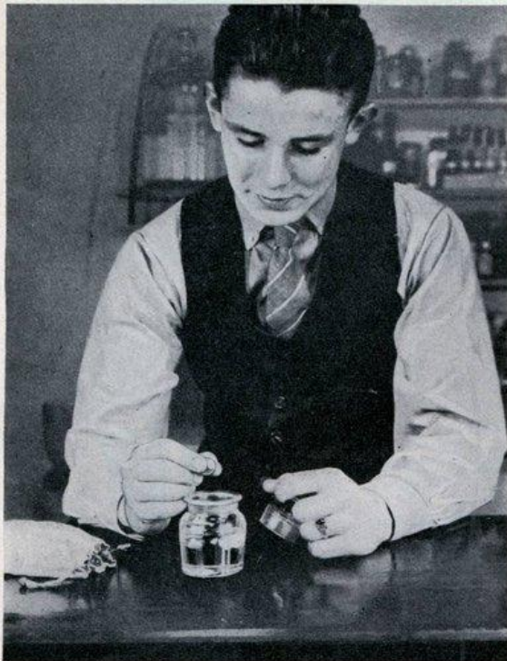
Glass marbles float in Thoulet's solution, which you can prepare by dissolving some red mercuric oxide in potassium iodide
