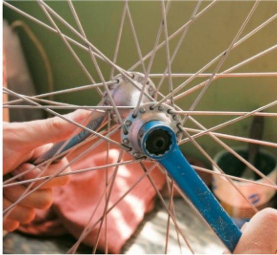
**Remove the outside locknuts using regular wrenches.**
