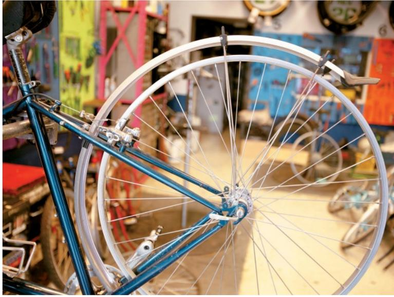
Plenty of fender clearance for a large tire on this bike.
