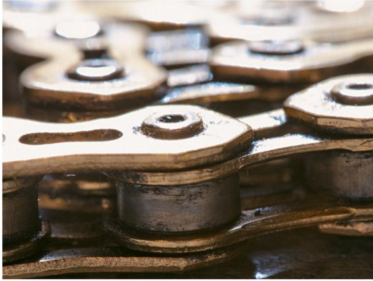
Bike chains are made up of a series of plates and rollers that spin around on your chainrings and cogs, pulling the back gears so that your rear wheel spins when you pedal. Your chain is one of the most important areas on your bike to keep lubricated; it moves quite a bit and rubs against a lot of other metal while being exposed to the elements.
