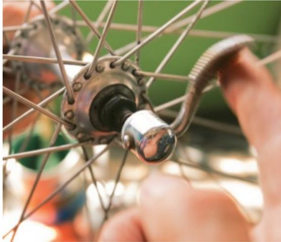
**Removing the quick-release skewer**
