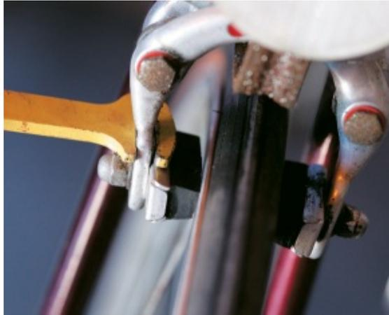
**Using a brake alignment tool on center pull brakes**
