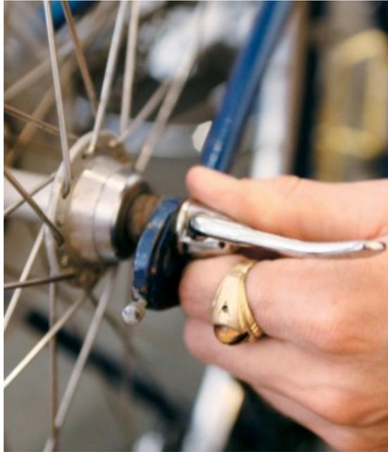
**Hold the level perpendicular to the frame and twist the nut on the opposite side snug before closing.**
