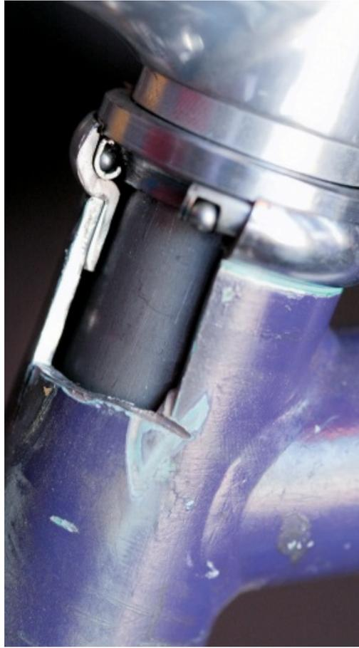
**Cutaway view of head tube and headset assembly**
