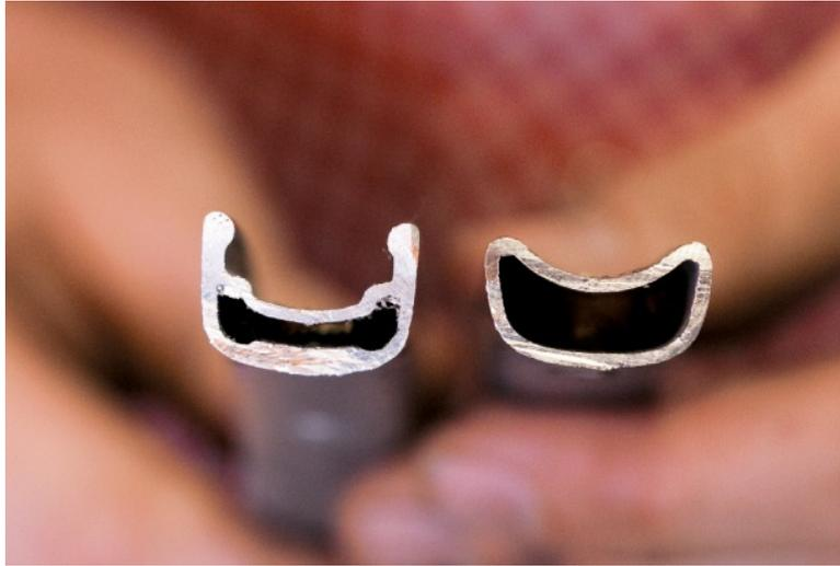
**Cross-section of rims: hooked, left; tubular, right**
