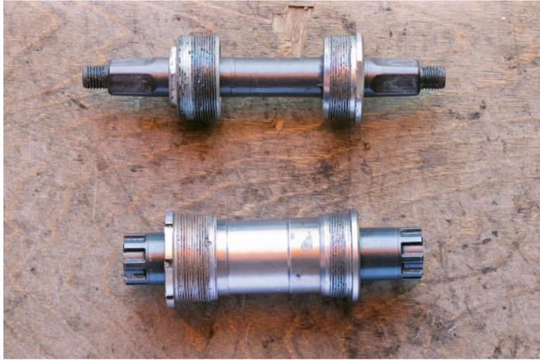
**Loose ball bottom bracket; bottom: sealed bottom bracket**
