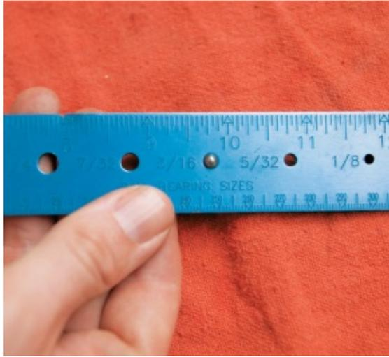
**You can always measure your bearings for replacement using the holes in a spoke ruler.**
