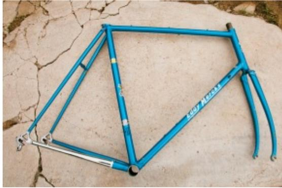
A more modern bare frame, this one comes with no bottom bracket or headset, meaning you should inspect it thoroughly before purchasing parts to ensure a match.
