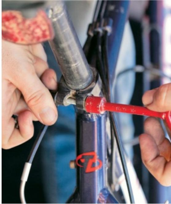
**Tighten the bolt down to hold your seat in place.**
