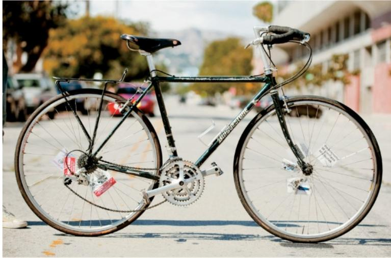
Seat tube angle is measured against the ground; a 90-degree seat tube would be completely vertical. The greater the seat tube angle, the closer it is to vertical, and the more it is considered to be an “aggressive” geometry. This is because a more vertical seat tube moves the rider farther forward over the pedals, which allows for great power in the downstroke, but is less comfortable.
