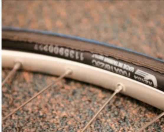
**The tube fits snugly inside the tire before being mounted on the rim.**
