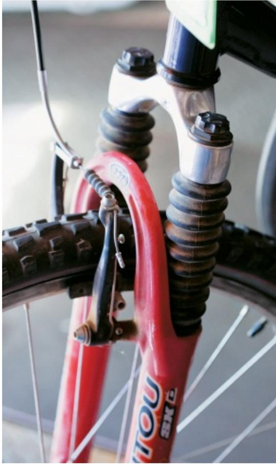
**Suspension fork with cantilever brakes on a mountain bike**
