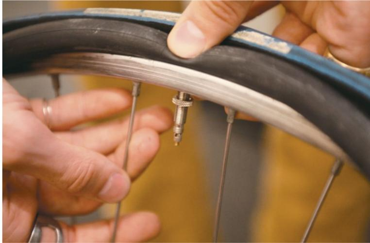
**Be sure to screw the locknut down completely on presta valve tires.**
