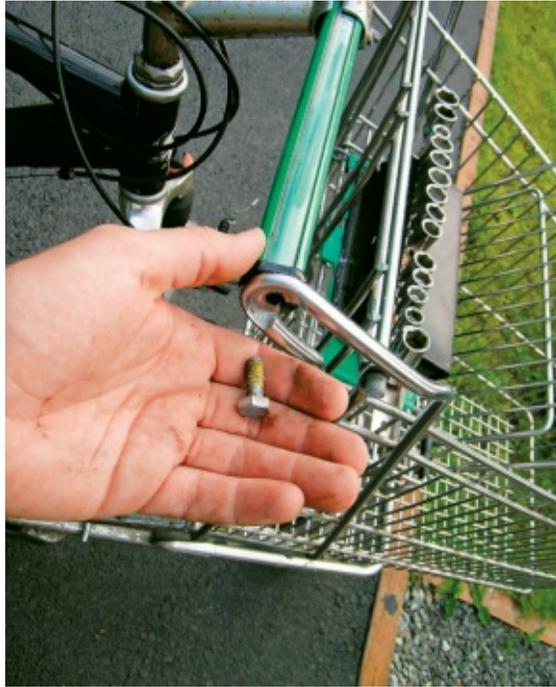
**Remove the screws holding the push bar onto the shopping cart.**
