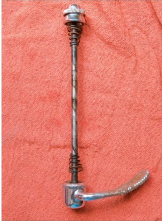
**Arrange your removed parts on a clean rag, in the order of removal.**
