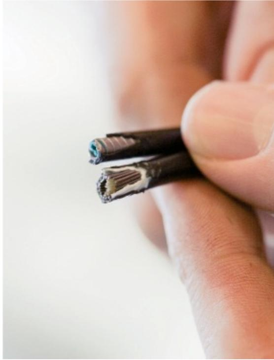
**brake cable; bottom: shifter cable**
