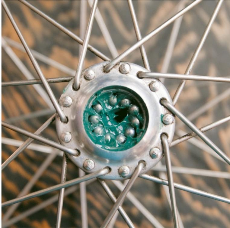
**The hub shell serves as the cup in the bearing assembly; the bearing cones are attached to the axle. The axle is a long threaded rod, and the cones are held in place using locknuts, which twist against the cones to hold them in place on the rod without tightening them down on the bearings.**
