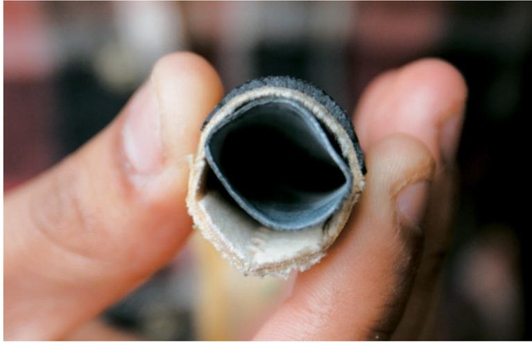
**Cross-section of a tubular tire**
