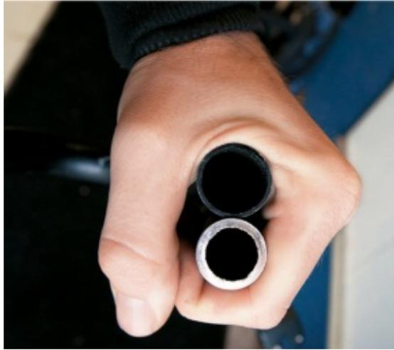
**Road bars have a thicker tube diameter than mountain bars, while in this case the mountain bar has thicker tube walls.**
