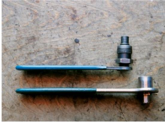
**Crank puller/crank bolt wrench**
