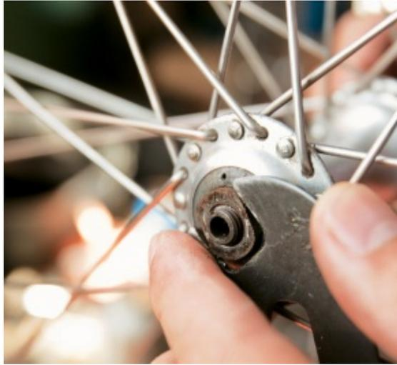
**Remove the cone nuts using flat wrenches.**
