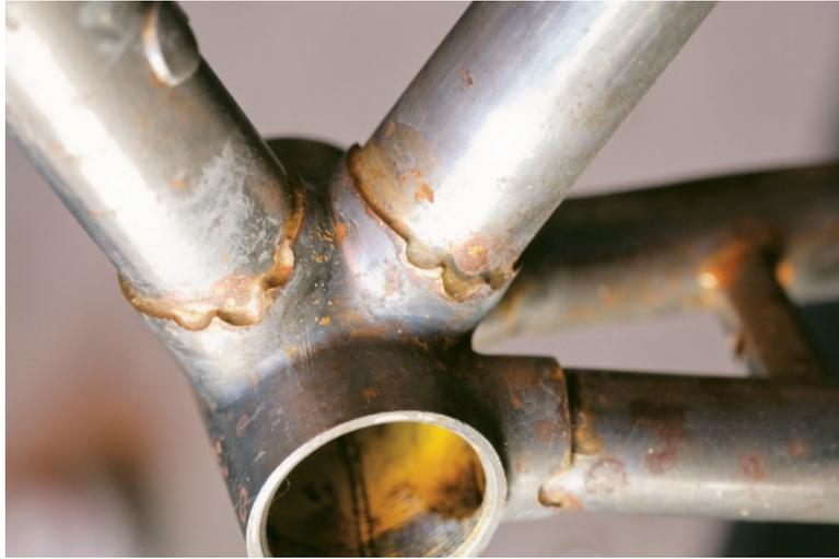
**A bottom bracket shell in a bare frame**
