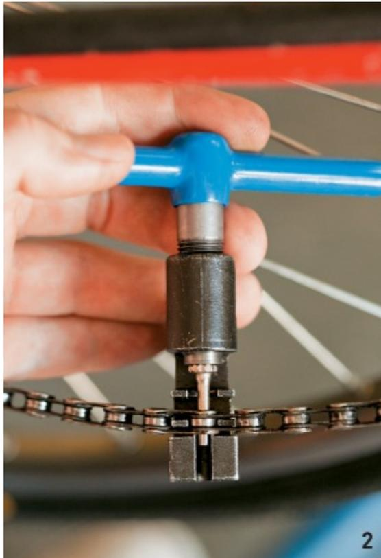
2. Slowly twist the handle to drive the pin into the chain, slowly pushing out the pin from inside the chain.
