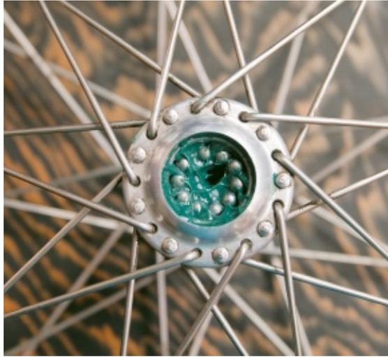
**Using grease to hold the bearings in place, replace the bearings in the hub.**
