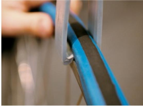
5. Once your bead is back on, fill the tire to the desired pressure, paying attention for bulges; if the wire bead isn't set properly, a section of the tire might bulge out. Inspect all the way around once you have filled your tire to ensure that the bead is properly seated on the rim. If it is not, your tire might not be compatible with your rim.
