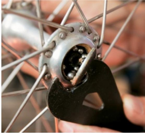
**Remove the dust cap, if necessary; many hubs do not have dust caps.**
