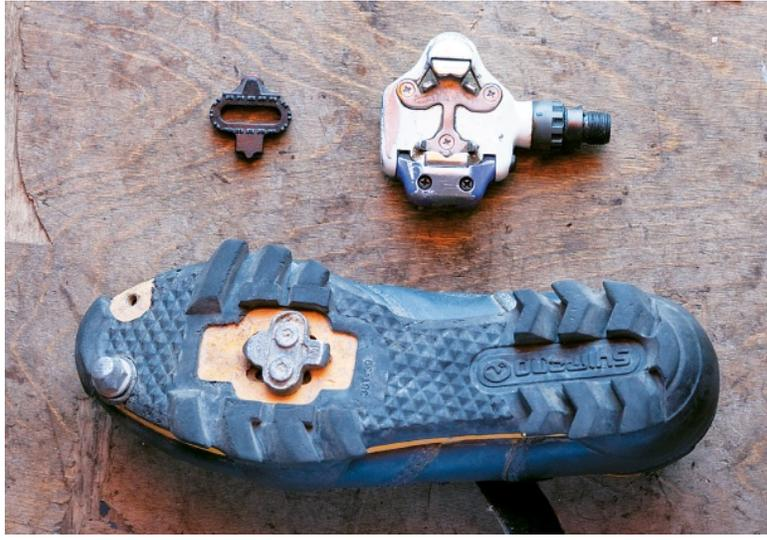
**Clips**, a newer system of keeping your foot on the pedal that became popular in the 1980s, are also known as clipless or cleats. These require you to wear special shoes with mounting points for cleats that clip into specially designed pedals that have a receiver for the toe clips.
