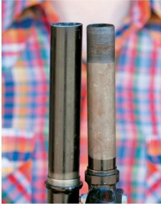
**Threaded and threadless steerer tubes**
