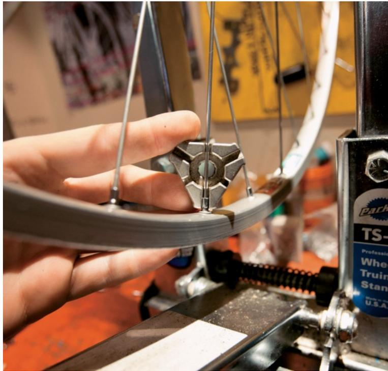
**Using a spoke wrench on the spoke nipple in the stand**
