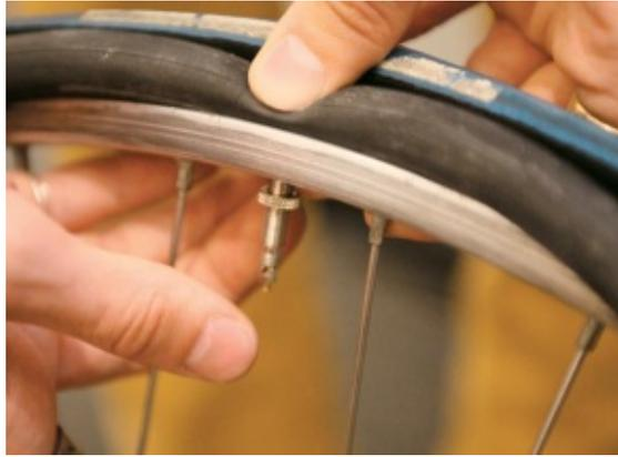
2. Next, tuck the lightly inflated tube into the tire all the way around.
