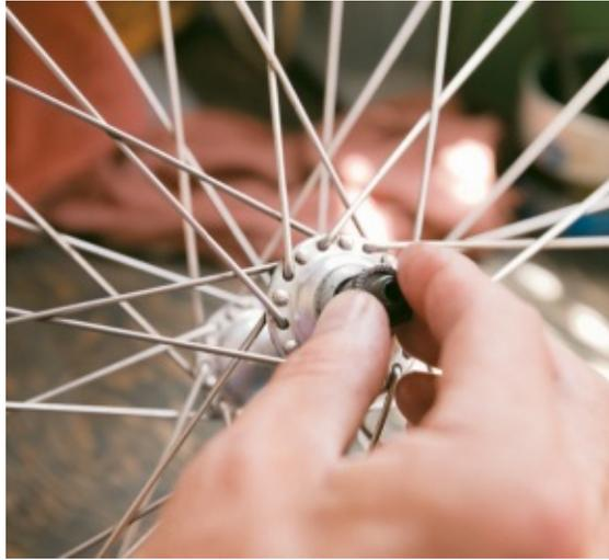
**Insert the axle and thread on the opposing cone nut by hand.**
