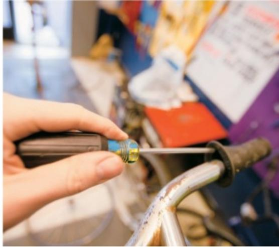
**A long, thin screwdriver is great for opening up a space to spray soapy water when removing grips, if necessary.**
