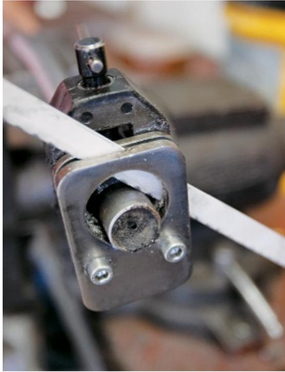
**Attaching a guide helps you keep your saw cut straight and level.**
