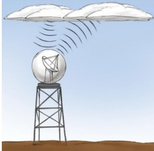
Radio transmitters use microwaves to detect precipitation intensity and locations.
