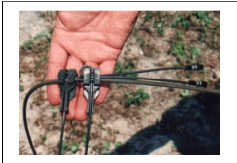
Figure 7-20. M11 or M16 branch lines connected to the detonating cord
