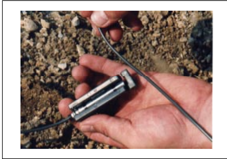
Figure 7-28. M15 25-millisecond delay blasting cap with a plastic connector
