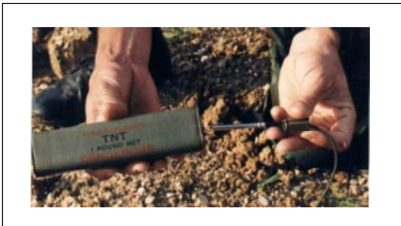
Figure 7-7. Priming TNT blocks with MDI
