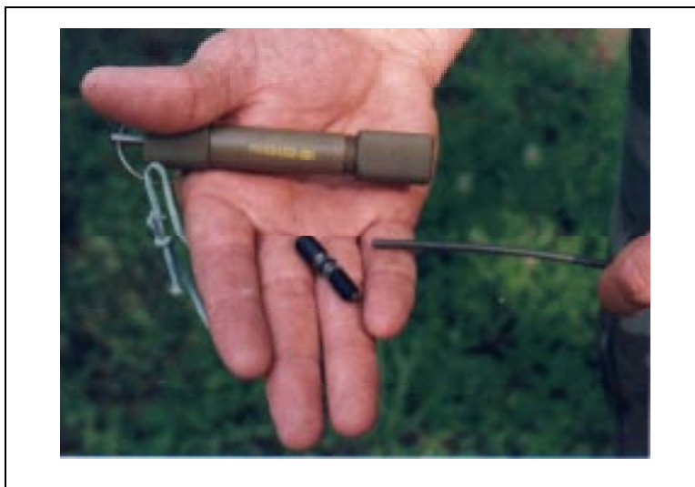
Figure 7-12. M81 fuse igniter with shock tube
