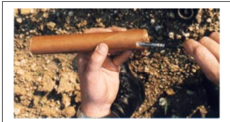
Figure 7-8. Priming M1 dynamite with MDI
