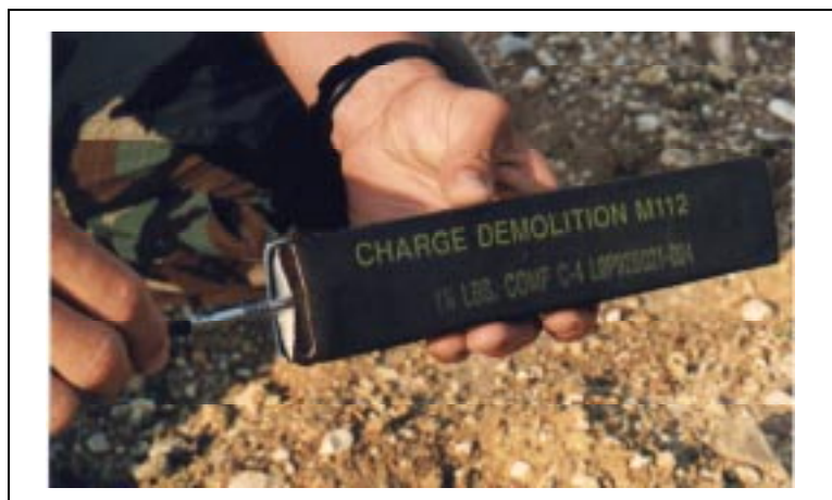
Figure 7-9. Priming C4 demolition blocks with MDI
