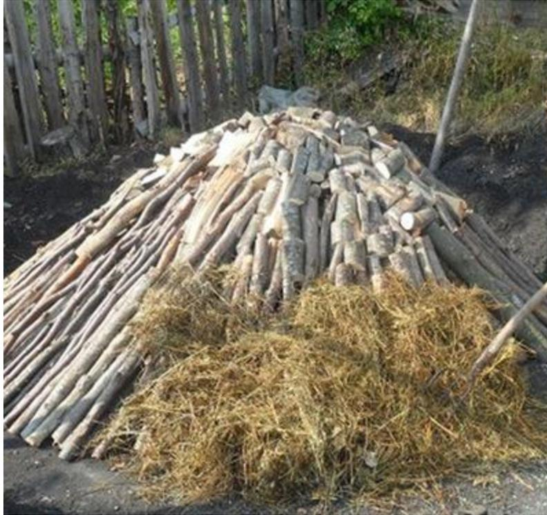
*“Over the entire pyre I put scrap pieces of coal that is left from previous productions or dry soil”.* According to Peter, the secret of coal quality is the wood burning and smoldering – as long as the wood used is neither too dry (in which case it burns too quickly) but not too green (in which case it would melt because of the heat).
